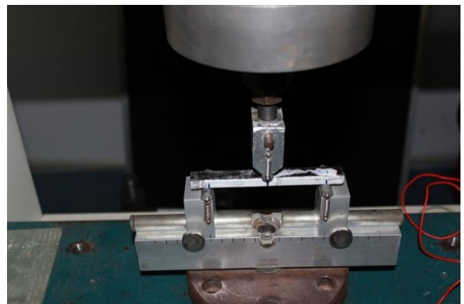
Figure-7 Three point bending arrangement
