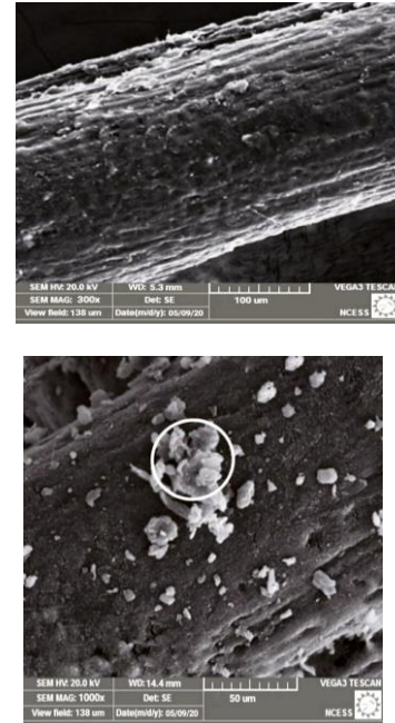
Fig. 2. Surface structure of coir fiber (a) unmodified (b) Ca(OH) 2 modified
